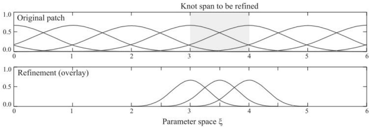
Figure 4: Refinement of a knot span [2]
