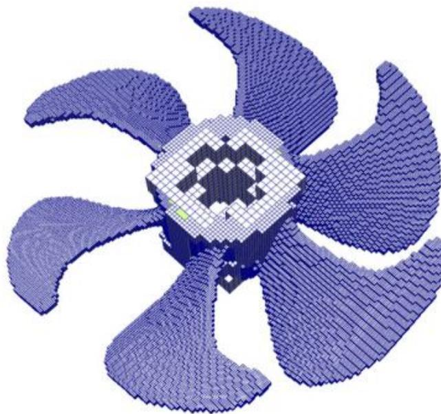
Figure 13: Sub-cell partitioning of the ship propeller (226.272 sub-cells of level  $k = 2$ ) [2]
