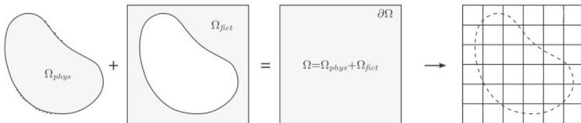
Figure 6: Embedding the original geometry into a larger domain of simple geometry [2]
