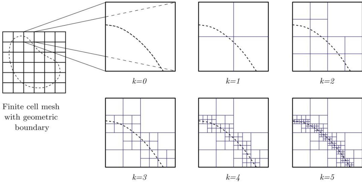
Figure 7: Hierarchical refinement on structured grid [2]
