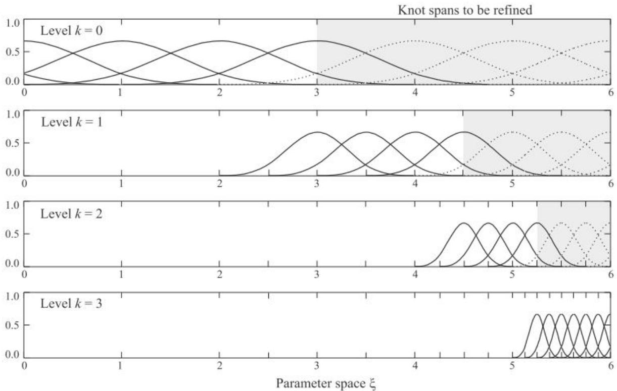
Figure 5: Hierarchical refinement scheme and removing basis functions (dotted lines) [2]
