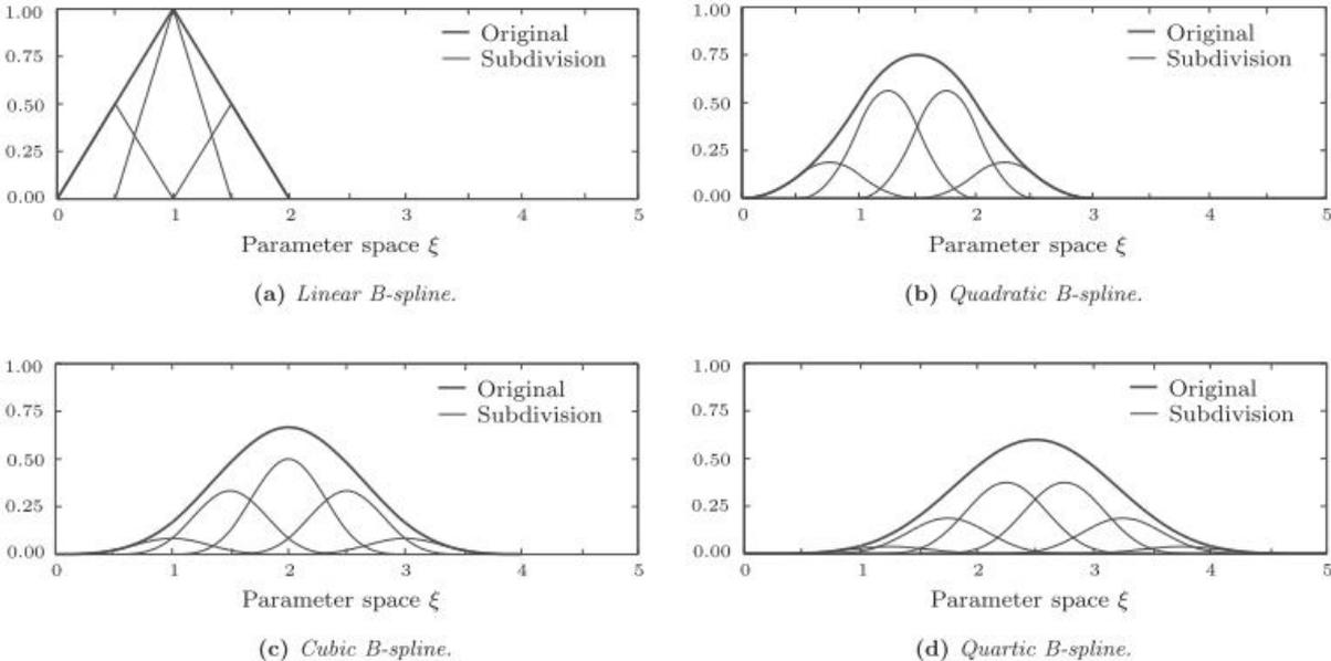
Figure 3: Subdivision of B-spline basis functions [2]
