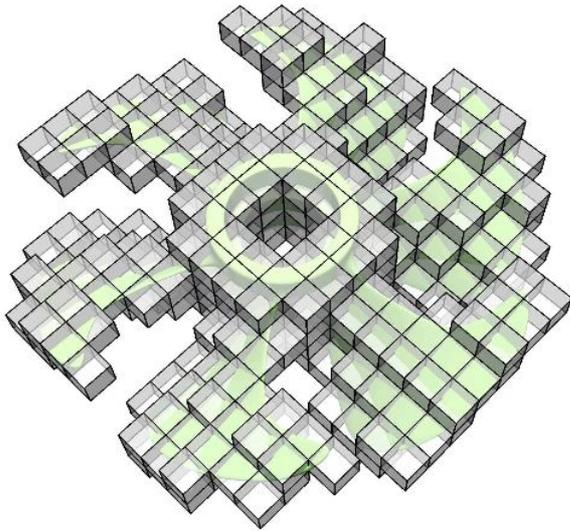
Figure 11: Deletion of cells without support in the propeller domain [2]
