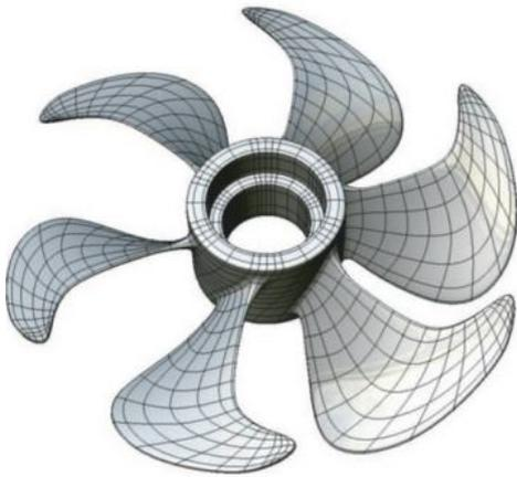
Figure 9: T-spline surface of a ship propeller [2]
