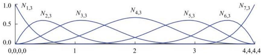
(a) Cubic B-spline patch with interpolatory ends.
