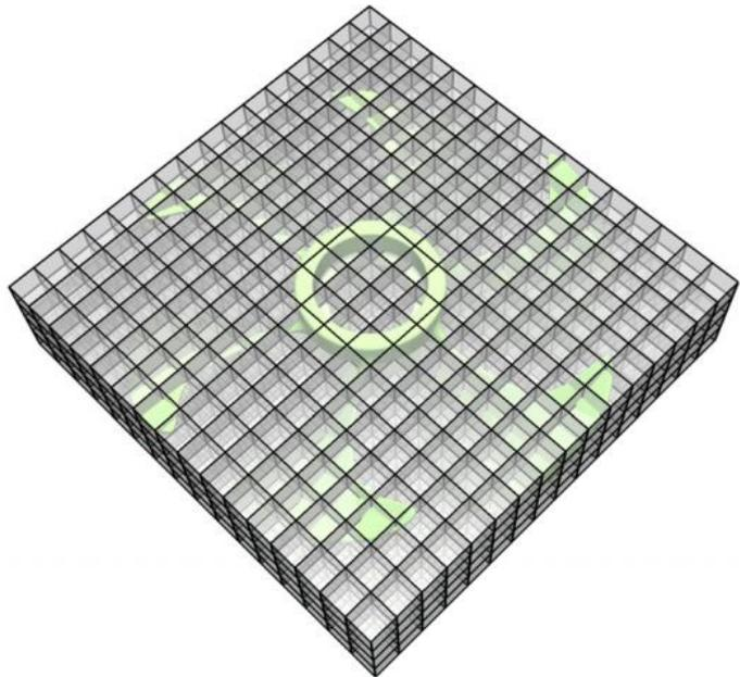
Figure 10: Propeller is immersed in a bounding box of B-spline elements [2]
