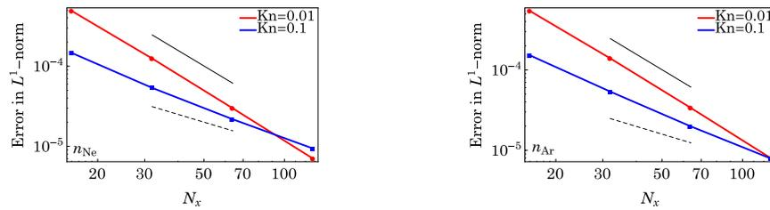
Figure 2: Empirical error in number densities of (left) Ne and (right) Ar in Ne–Ar mixture for different Knudsen numbers. The continuous and dashed black lines have the slopes of  $-2$  and  $-1$ , respectively.
