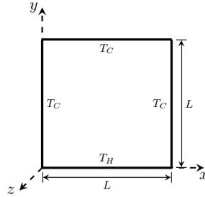
Figure 1: Schematic of a two-dimensional bottom heated square cavity;  $T_H > T_C$ .
