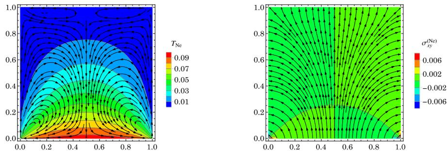
Figure 3: (Left) Velocity streamlines and temperature contours (right) heat flux lines and shear stress contours for Ne at  $Kn = 0.01$ .
